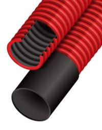
Super Corflo is a dual-wall coilable polyolefin duct, and is the economical choice for conduit and inner duct applications. The dual-wall design offers a light-weight, easy to handle conduit system with an increased crush-resistance, and semi-smooth inner wall for ease of cable pulling. Super Corflo® can be used anywhere Rigid PVC is used: Inner City work (structures), Solar Farms, or any Open Trench work.
